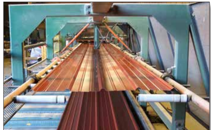
Wall and roof steel roll former up to 48' length
